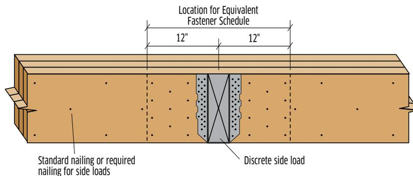
**Example:** Assuming a properly designed 3-ply 14" beam, determine the equivalent connection to support a factored point load of 6970 lb applied to the side of the beam.
